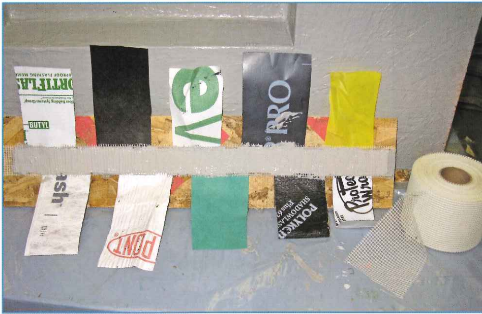
Photo 22 – Tie-in to sheet WRBs and flashings made easy.
