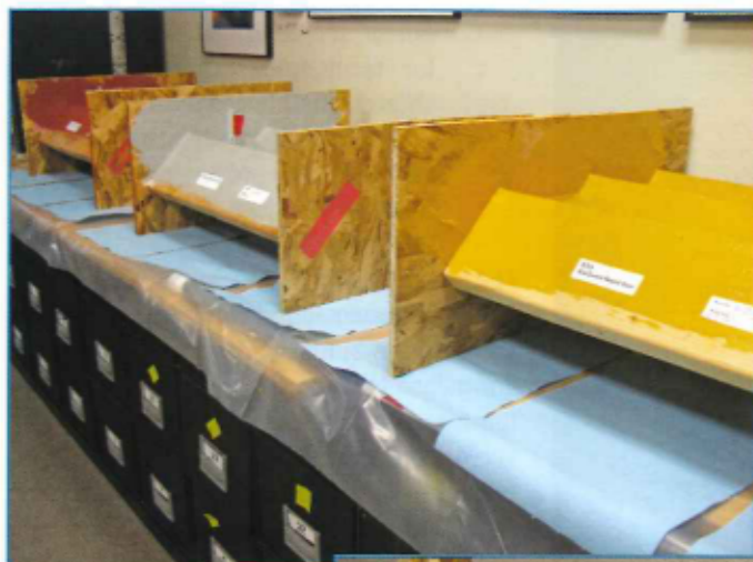
Photo 19 – In-house seven-day flood testing of fluid-applied flashings.
