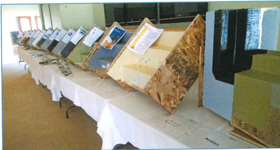
Photo 24 – The author applied 15 different manufacturers’ “paint-on flashings” to mock-ups for the 2014 Westcon Symposium and 2015 RCI SoCal Hawaii Winter Workshop presentations.
